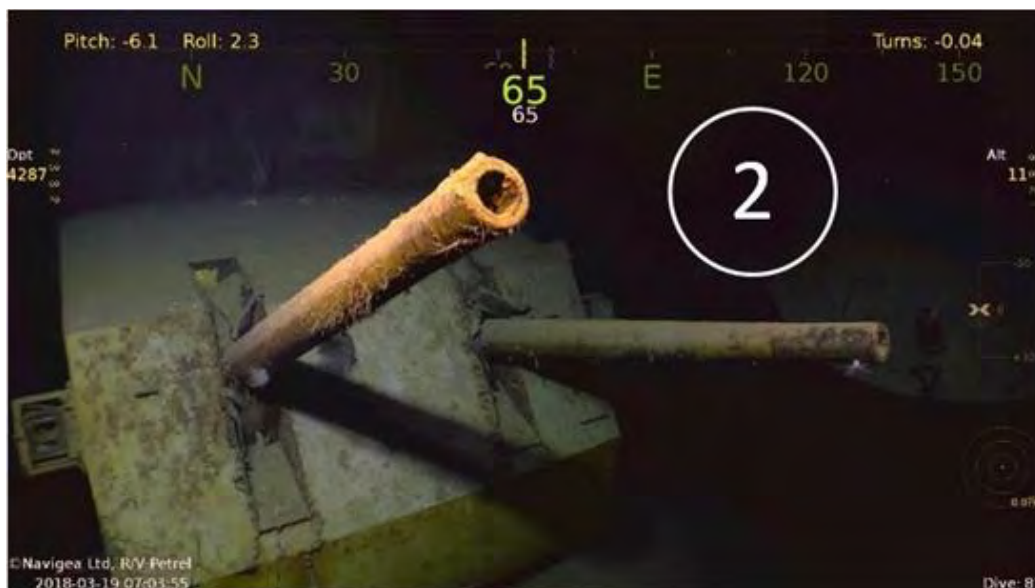
Starboard side 5-inch gun mount (turret no. 5). The transverse crack in the Juneau ’s deck developed behind this turret. Photo reprinted with the permission of Vulcan, Inc.
