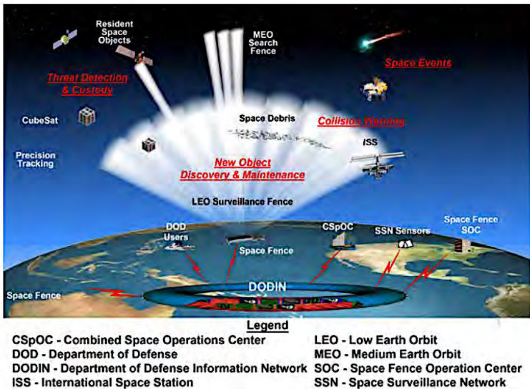
Figure 3. Components of the Space Fence
